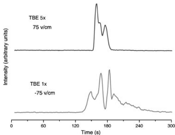
**Figure 4.** Electropherograms measured at 1 cm in a  $d_s = d_d = 80$  nm device.
