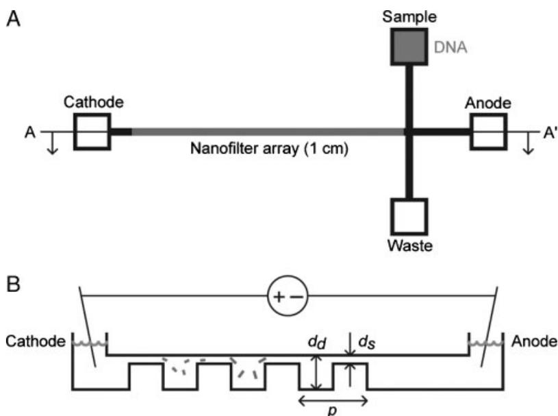
**Figure 1.** Schematic of the nanofilter array. (A) Device layout. (B) Schematic cross-section through A–A'. An electric field in the nanofilter region causes shorter DNA molecules to travel faster.
