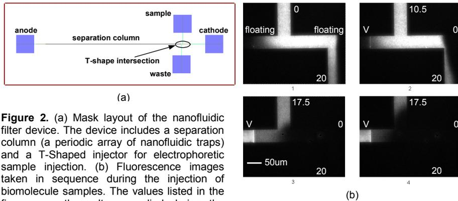
**Figure 2.** (a) Mask layout of the nanofluidic filter device. The device includes a separation column (a periodic array of nanofluidic traps) and a T-Shaped injector for electrophoretic sample injection. (b) Fluorescence images taken in sequence during the injection of biomolecule samples. The values listed in the figures are the voltage applied during the injection in all our experiments.
