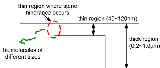
**Figure 1.** Cross-sectional schematic picture of one nanofluidic trap. When molecules travel through the thin region, certain configuration entropy will be lost due to steric constraints imposed from the walls. The entropic free energy barrier caused by this will slow down the motion of molecules and induce the size dependence of electrophoretic mobility in the nanofluidic filter.
