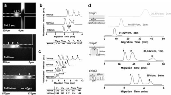
Fig. 2. a, Sequence of fluorescence images showing separation of the SDS-protein complexes (1: cholera toxin subunit B, 11.4 kDa; 2: lectin phytohemagglutinin-L, 120 kDa; 3: low density human lipoprotein, 179 kDa with  $E_{av}=100$  V/cm. b-c, Separation of SDS-protein complexes (b) and dsDNA molecules (c) under different applied fields. Band assignment for DNA: (1) 50 bp; (2) 150 bp; (3) 300 bp; (4) 500 bp; (5) 766 bp. d, Comparison of three different nanofilter array devices.
