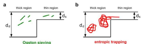
Fig. 1. Ogston sieving (a) and entropic trapping (b) of biomolecules across a nanofilter.
