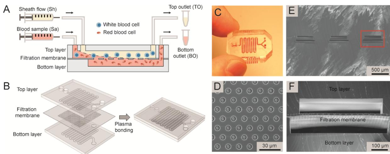
Figure 1: Continuous-flow microfluidic cell sorting using crossflow filtration with PDMS microfiltration membranes (PMMs).
